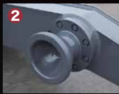
Grip Rotates objects forwards or backwards that are grabbed by the clamp
