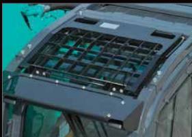
Standard Overhead Top Guard Level II The standard overhead cab guard can be tilted open for easy window cleaning.
